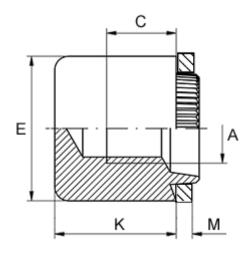
Female thread A = M4Height K = 9.0Min thread length C = 4.0Outer diameter E = 10.0Plate thickness = 2.3 to 2.5
